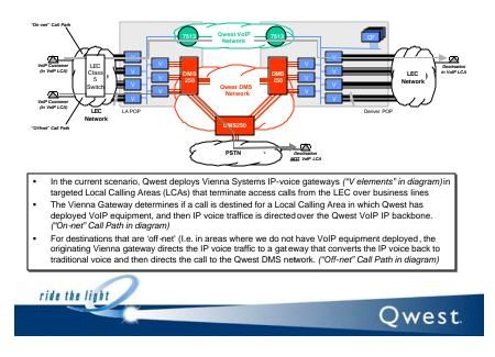
Figure 7-2: Example of VoIP Application (Source Qwest.com)
