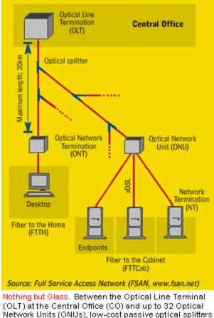
distribute optical signals without requiring electricity.
