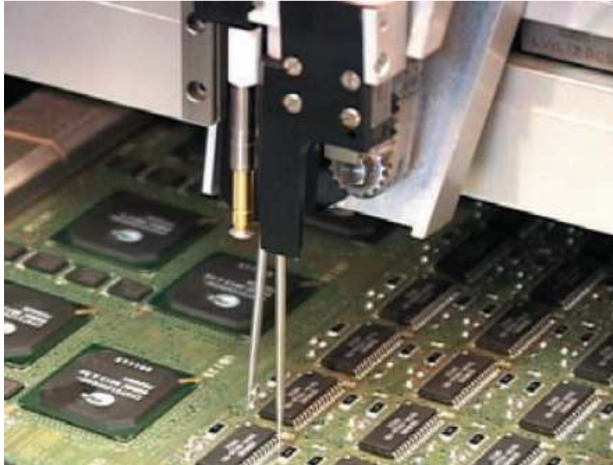
Figure 12. Flying Probe Testing a Printed Circuit Card
