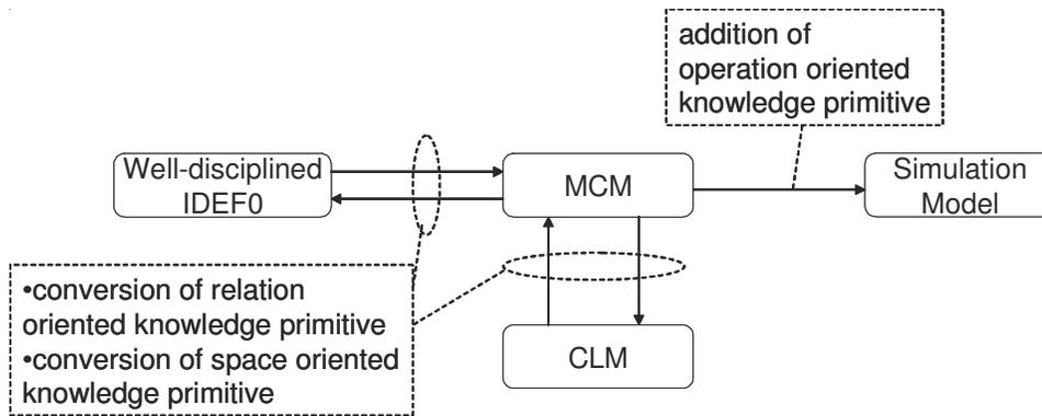
**Fig. 13 Conversions Between Well-disciplined IDEF0, MCM, CLM and Simulation Model.**
