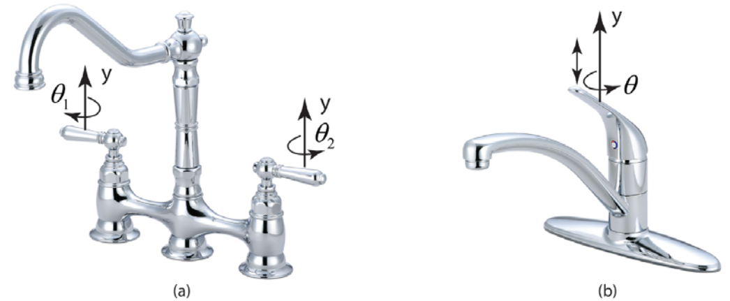
Figure 6.4: (a) Two-handed water faucet, (b) One-handed water faucet. (Adapted from Frederickson B., 1994, Holistic Systems Engineering in Product Development, in Saab-Scania Griffin, vol. 1994/95, Linköping, Sweden: Saab-Scania AB, S-581 88, pp. 23-31, 1994).
