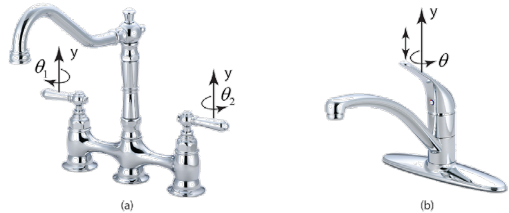
Figure 6.4: (a) Two-handed water faucet, (b) One-handed water faucet. (Adapted from Frederickson B., 1994, Holistic Systems Engineering in Product Development, in Saab-Scania Griffin, vol. 1994/95, Linköping, Sweden: Saab-Scania AB, S-581 88, pp. 23-31, 1994).
